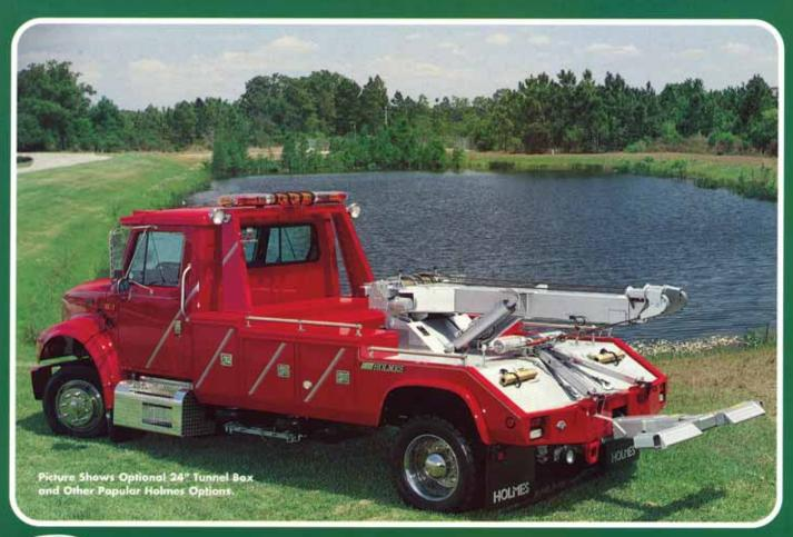
esigned for the operator who wants to step beyond a light duty chassis, the Holmes HP 552 is a towing and recovery unit that will provide years of tough, dependable service. The 552 is equipped with the LD 6500 underlift, a twelve-ton recovery boom, and winches rated at 15,000 lbs.
