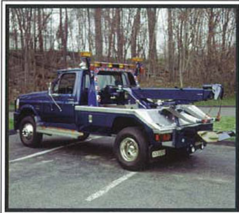
Century's optional aluminum Formula 1 body is constructed using a steel subframe and tailboard, shiny diamond aluminum floor plate, polished aluminum extrusion top rails, aluminum side panels and tool compartment.
