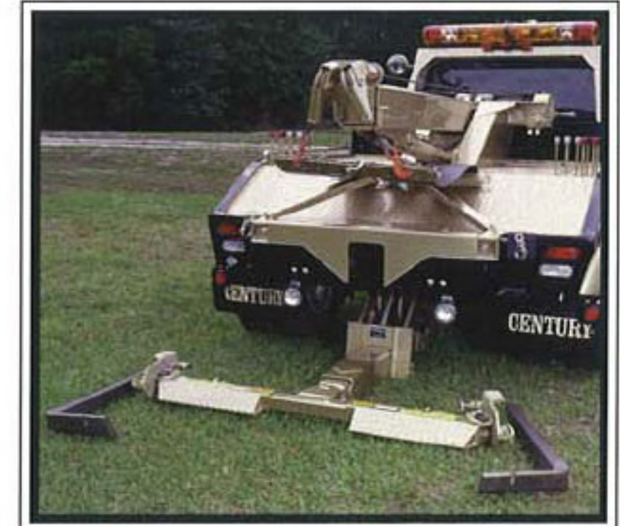
Century's pivoting L-arm system provides for fast, efficient and safe hookups. A centering pin lines the lightweight L-arm up with the camlock for a fast connection. By removing a pin, the L-arm end castings may be swiveled in or out to be positioned with the tires, even when the wheels are turned.
