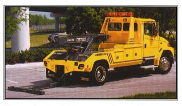
The Formula II T underlift is constructed using a fabricated inner stinger for added strength while still maintaining a low profile. The twin tilt cylinders provide a total range of 22° positive and negative tilt.
