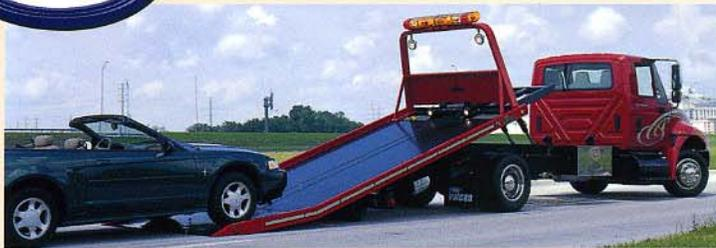
← Throw away the wood planks and ramps, simply release the bed lock and the rear deck section hinges down to a 6° load angle for low clearance vehicles.
