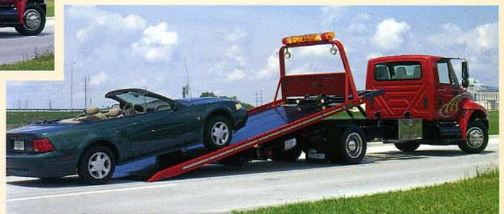
For low clearance rear bumpers or exhausts the rear deck can be lowered a second time for increased rear clearance while completing the loading or unloading process. →
